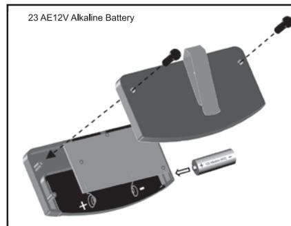
Replacing Transmitter Battery:
