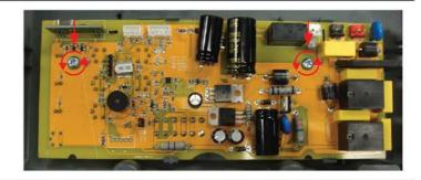
4. Release the logic board from the panel by pressing on the plastic clips at the edges of the board, one side at a time. Be careful not to break the clips.
