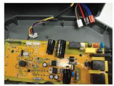
3. Remove the two silver screws in the logic board.
