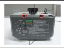
2. Unplug the leads from the motor that are connected to the logic board.
